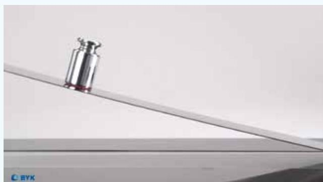
Demonstration of increasing and reducing surface slip
